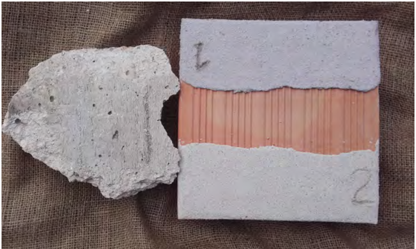
The identification of the repair mortar; two tests, compared to a sample of original material. 2
