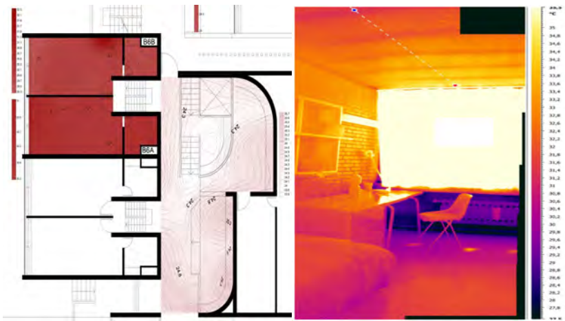
Figure 9. Distribution of temperature (left) in B6b room (top) and B6a (bottom) compared with the common space (in the middle) of the building "Aquilone" – 14/07/2016. Thermal image of B6b room - 14/07/2016 (right).
